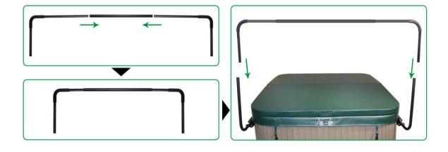
Step 3: Lay the Cover Lift on the spa cover. Position ①, using the Self Tapping Screws to fasten the Support Arms and Coupler Piece together. Position ②, using the Self Tapping Screws to fasten the Support Arms to the Pivot Arms. Then press the decorative Small Black Dome Caps over the heads of all the exposed screws.
